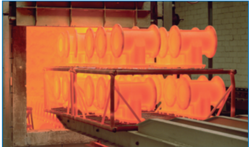
Multamed Gate Valve bodies after the annealing process
