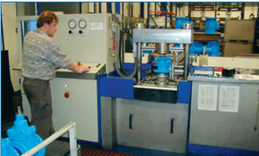
Testing of Multamed Gate Valves at the factory
